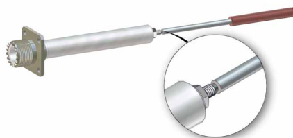
Solder contact (8) on conductor.
